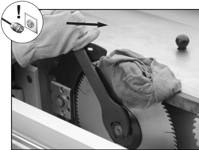
Figure 82. Removing arbor nut to change blade.
